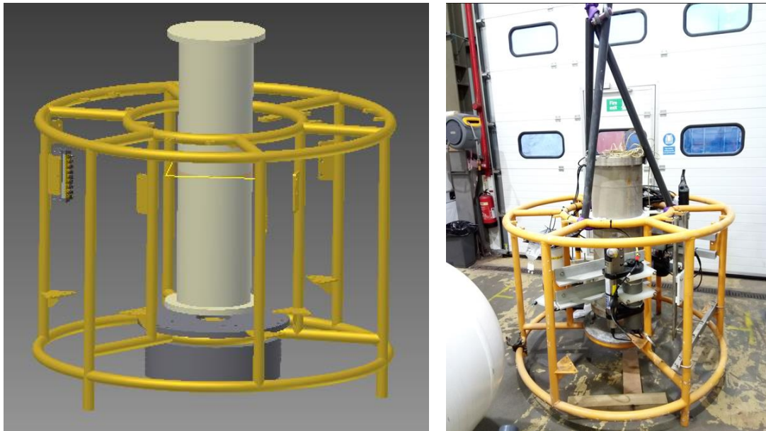
Figure 5-22 Schematics of the lander design (left) an image of the lander with sensors (right). The central white tube contains the battery.
